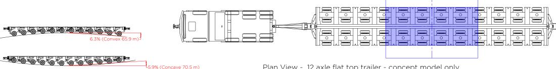
Vertical Curve Negotiabilty Information based on manufacturers literature Scale: 1:300 Plan View - 12 axle flat top trailer - concept model only Indicative 157 te transformer Scale 1:150
