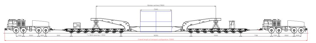
Elevation view - 16-axle girder frame trailer - concept model only Indicative 157 te transformer Scale 1:250
